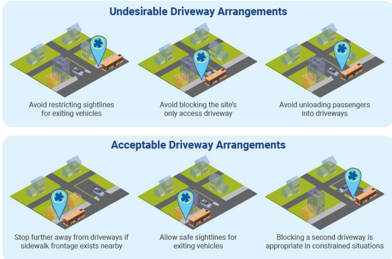
FIGURE 26: RECOMMENDATIONS FOR POSITIONING BUS STOPS AROUND DRIVEWAYS
