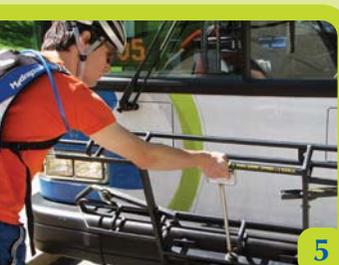
*After removing bike, raise and secure rack if there are no other bikes on rack.*
